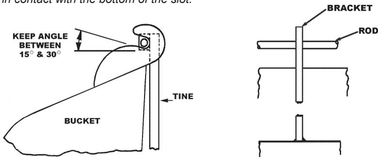
*If the top of the bucket is curved or there are stiffening members along the top, trim the bottom of Mounting Brackets to fit the contour of the bucket without having a gap exceeding 1/8". The Mounting Brackets must be mounted perpendicular to the top of the bucket.*
