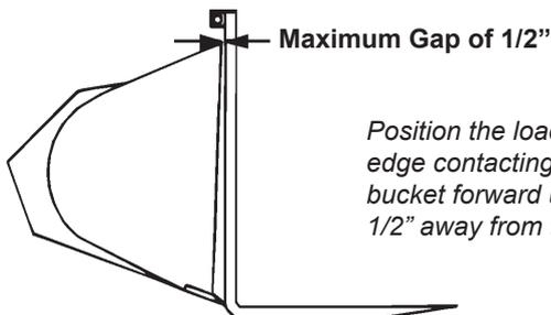
*Position the loader bucket so that the cutting edge contacting the back of the fork tine, roll the bucket forward until the spill guard is roughly 1/2" away from the back of the fork tine.*
